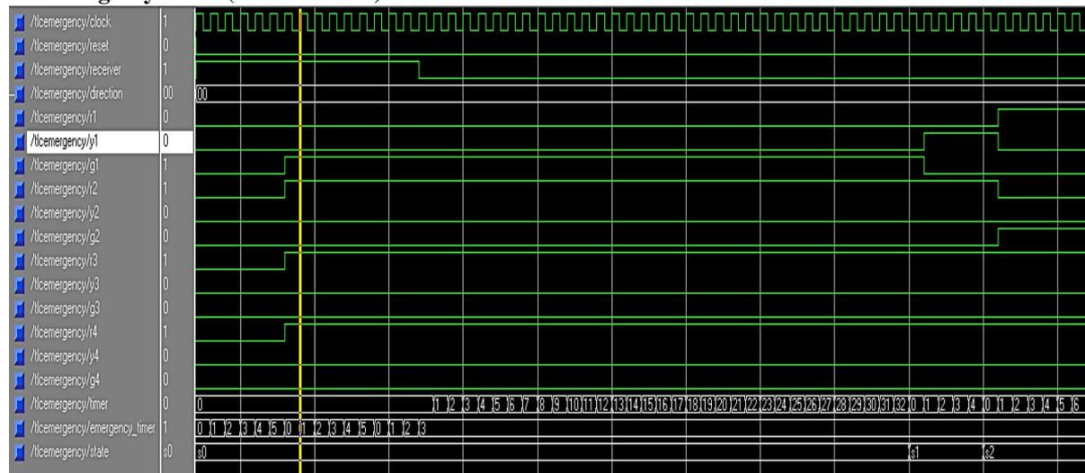
Fig(6). Simulation of emergency sequence mode for direction=00
