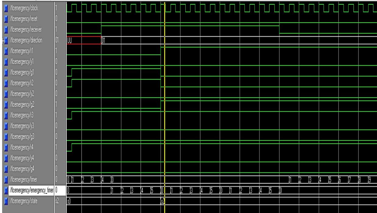
**Fig(7).** Simulation of emergency sequence mode for direction=01
