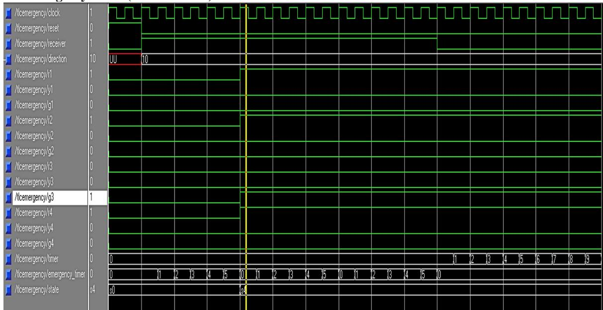
**Fig(8).** Simulation of emergency sequence mode for direction=10
