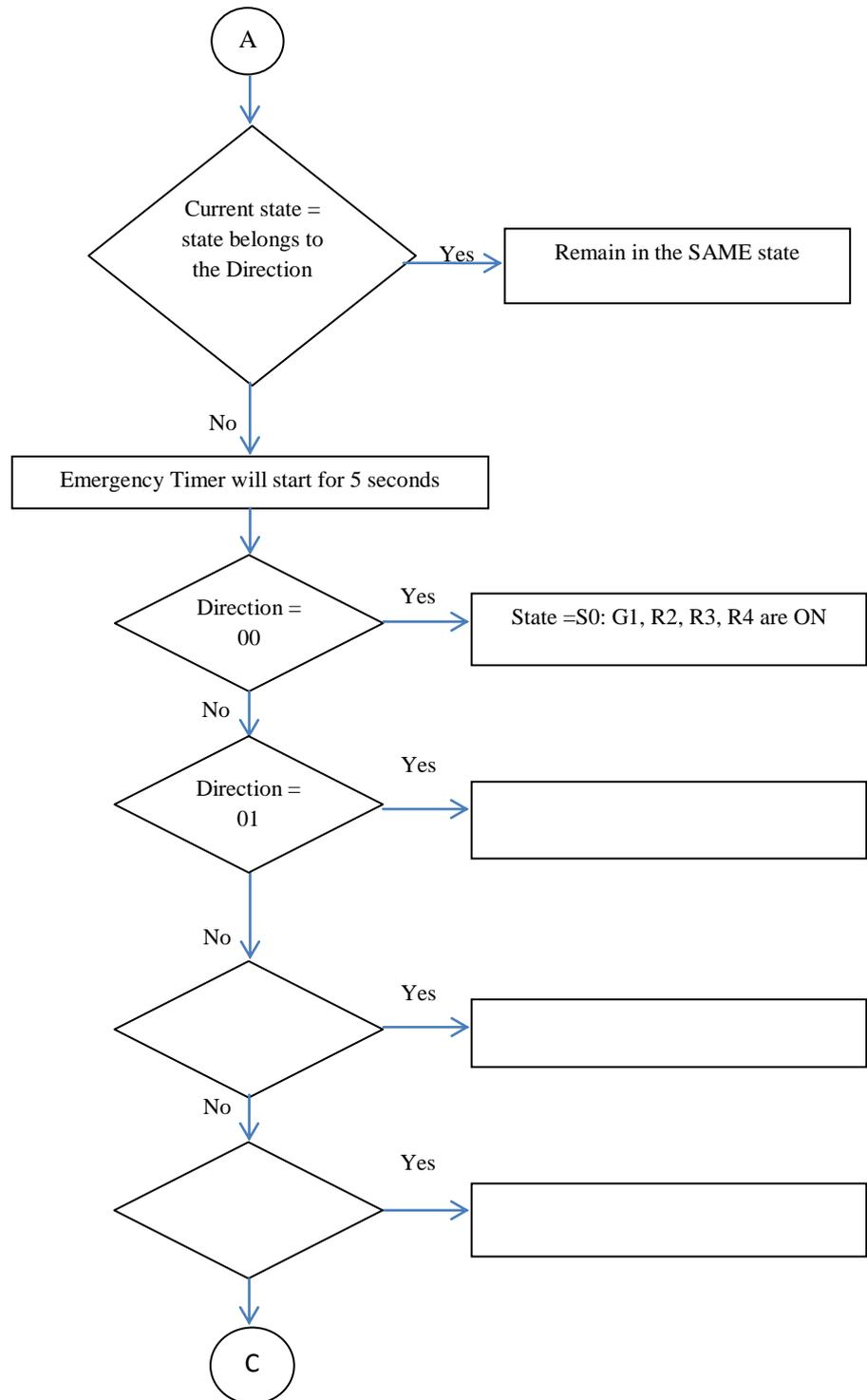
**Fig(4).** Flowchart for emergency sequence mode.
