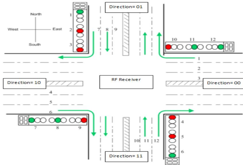
Fig(1). Four way traffic light system
