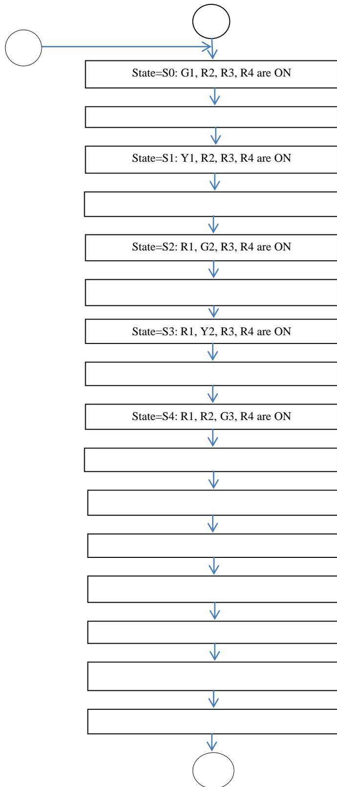
Fig(3). Flowchart for normal sequence mode.
