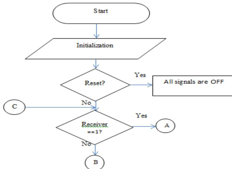
Fig(2). Flowchart for how system detects emergency condition.
